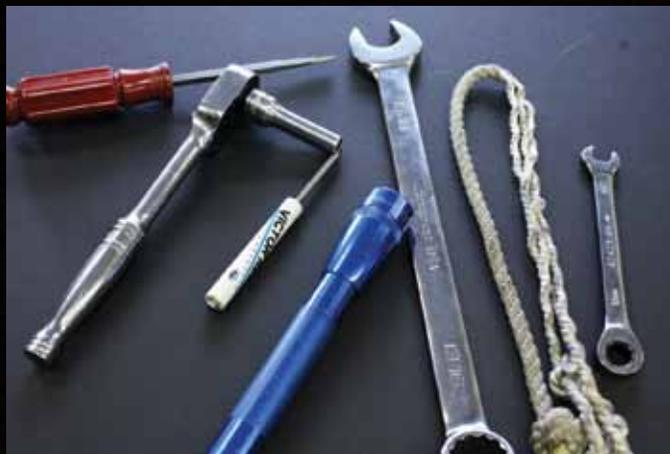
necessary to replace your valve springs without removing the cylinder head.
