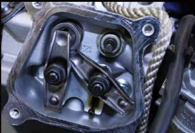
new one. Reverse the procedure to reconnect the valve. Move the rocker arm back into position by pushing down on the valve and rotating the rocker arm back into position. If you removed it completely, replace and reset the valve lash. Repeat the procedure for the other valve, being sure to reinstall the lash cap on the exhaust valve.
