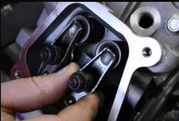
one of the rockers, let's start with the exhaust, and sweep left to right over the tip of the valve. You should feel a slight bit of friction, but no tension as you sweep across. There should be no upward movement on rocker arm either. Use a feeler gauge if necessary to determine if you have too much lash, if it fits, it's too much lash.
