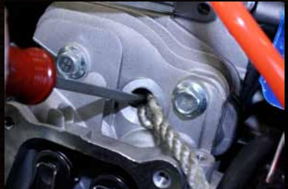
is to hold the valves in position so once we unhook the retainers it will keep them from dropping into the cylinder. You can check yourself by pushing down on the valve, if it moves downward over 1/8" or so, you may need more rope.
