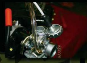
a regular basis. Use a quality filter that you can see through, this will help you know when replacement is needed. Occasionally it is advisable to remove the floor tank and clean it out as well. Just use a keen eye and good judgment here. Inspect your fuel lines as well, alcohol tends to dry and make them stiff, and sometimes this can lead to air leaks. Replace as needed. Always use a zip- tie at all connection points to keep the lines from disconnecting.
