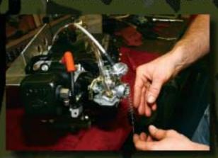
While spraying, shoot a bit into the earb and lubricate the slide. Sometimes is is a good idea to remove the slide to properly lubricate it and keep it from sticking. Just unserew the eap on the very top of the earb, and lift the slide out. Lubricate it and the bore it rides in and replace. Pay attention when re-installing the slide, as it is possible to install wrong. The side with the open slot all the
