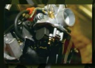
way down faces the header side of the engine. Work the throttle a few times and you are set. If you like, a little WD-40 sprayed on and around the jets is ok, however, do not do it in excess. Place the float bowl o-ring in its groove, and re-install the float bowl.
