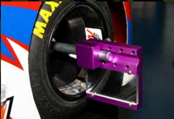
Opening the fitted case, you will see the components that make up the Accutoe pro kit. You will have the laser assembly, the rear axle laser bracket, and the thumbscrew to attach the laser to the bracket, and the mirror bracket for the front. I find it is necessary to have the expansion kit as well, as this gives you options as to the use of this instrument, whether you choose to use it
