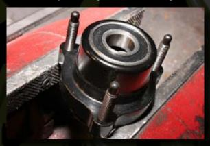
is a problem. As far as I am concerned, any bearing making noise is an issue, regardless of how free it appears to spin. Dirt and grit inside the bearing is the main cause of this. More often than not, a noisy bearing cannot be cleaned and oiled back to health and needs replacement. Any movement between the inner and outer race of a bearing is also a sure sign that it needs replacing.
