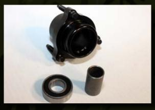
into the counterbore. If either of the bearings are cocked, the inner races will not be parallel and the hub will not slide freely onto the spindle arm. If this problem arises, make sure each bearing is fully seated.
