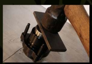
usually separated by a spacer to spread the load between both bearings. Remove the hubs from the kart and open a bench vise just enough to catch the outer edges of the hub on top of the jaws. Take a pin punch or other blunt object, and through the bore of the top bearing, drive the lower bearing out of the hub. Turn the hub over and repeat, and you should have a bare hub. Keep track of your inner spacer if so equipped.
