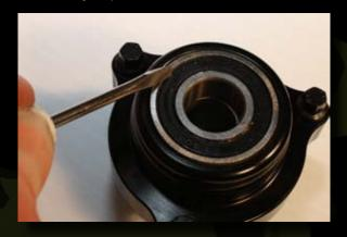
only way to clean, flush, and oil the bearings is to remove the metal dust cover and add a removable bearing shield. Bending the dust cover, or prying it away to add oil, will allow dust and dirt to enter and the oil to escape. The way I see it, you have two choices, either replace the bearings on a regular basis, or add the shields, any other method of maintenance for the axle bearings will be short lived at best. Since we are replacing bearings, let me add a cou-
