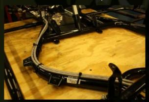
the bottom of the frame are at the same point. Using this as a base not only helps hold the seat in position, but it allows us to set the seat as low in the frame as we can without going lower than the frame and risk dragging the track.
