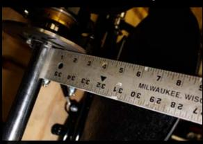
rubber washers at the contact points and washers under the bolt heads. Tighten by hand until the locknut makes contact. Do not over-tighten the seat, we want the seat to be free, not loose. Now, tighten the seat struts and the seat slides securely to the frame. Voila, one seat mounted and ready for action.
