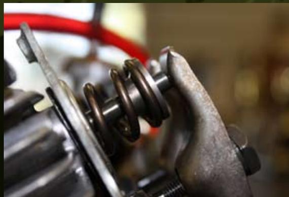
on the base circle of the cam and not the lobe. Rotate the engine slowly, looking down the spark plug hole with a flashlight, and turn until the piston is at the top of the cylinder and both pushrods down.
