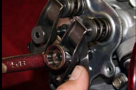
which they were removed. Parts that look the same sometimes have slight differences that can affect performance and sometimes tech. If disassembling for any reason, always separate the exhaust valve parts from the intake side parts. Always mark the pieces for the appropriate valve, and store separately.
