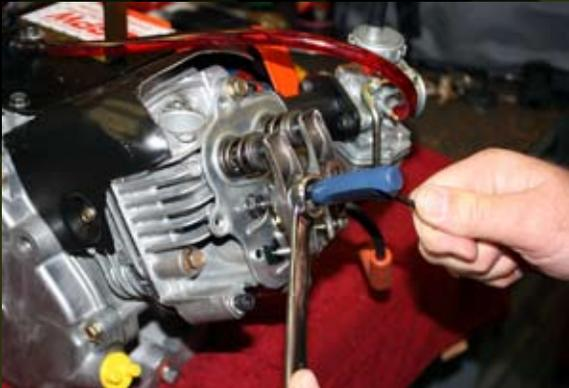
turn. Then, tighten it back with the 5/8 wrench until the lash is back at the desired setting. This will put more tension on the lock screw and help keep it from loosening up. Be cautious not to put too much tension on it, as the rocker stud can possibly break.
