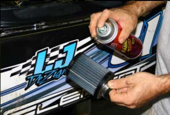
Use a quality filter and ALWAYS spray with filter oil. Carefully spray the filter and cover the filter area with a good even coat, wipe the excess off and you are ready to install. This will help keep dirt from entering the carb. Having a extra filter to replace at the track is a good idea. You can pre-oil the filter and store in a zip-lock bag. This helps save a step at the track.
