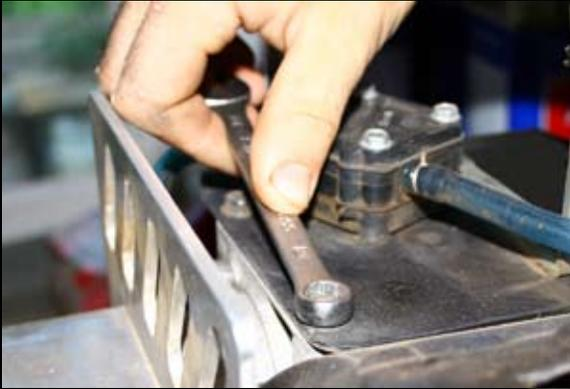
make sure everything is nice and tight. The main areas to check are the carb and tank bolts, and the header and header brace bolts. Head bolts and sidecover bolts should only be tightened with a torque wrench. Tight is tight enough, more than that can cause damage and break parts.
